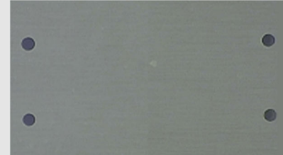
Ø0.15 Drill machining (x60) Zirconia (ZrO 2 )
